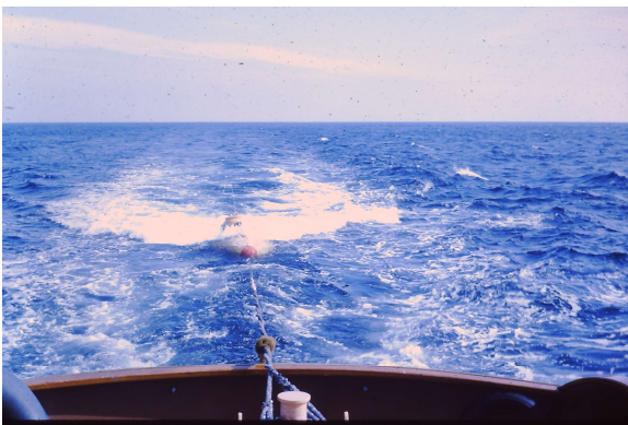
Submaray under tow with the towing pennant and towing bridle
