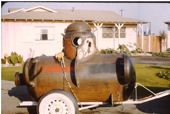
Initially Dolphin had ballast tanks on the side but that was scrapped for front and back cones. (Remember the sinking of the Sportsman Dry Sub, due to a lack of stability)
