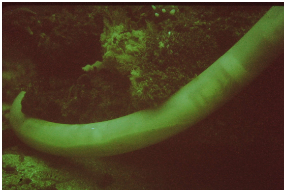
The seismic streamer stuck under a shale outcrop
