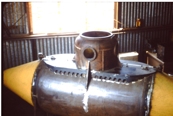
Dolphin with the front and back ballast tank cones installed.
