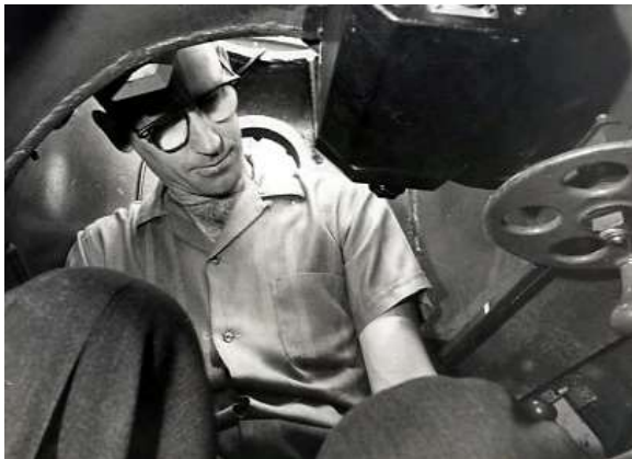
The rudder control (horizontal wheel) that was turned with your left hand
